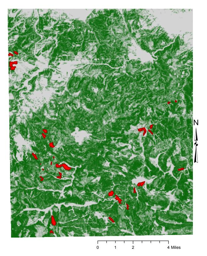
Suitable areas are determined by intersecting locations: Aspen Stands Low Infiltration Geological Substrates Within 500 Meters of a Primary or Secondary Road
